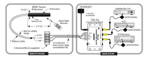
While it is possible to make wired connections without the connecting block, it is not recommended. The connecting block reduces installation time, helps to eliminate errors, allows easy troubleshooting and permits easy system upgrades later, if needed.
